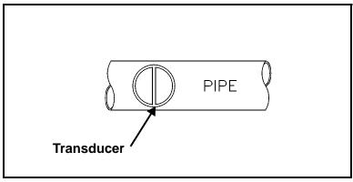
Figure C-1: Proper Alignment of Transducers for Cylindrical Surfaces
